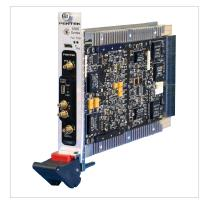
The 52741 is a high-speed data converter with a programmable DDC, suitable for connection to HF or IF ports of a communications or radar system. Its built-in data capture features offer an ideal turnkey solution.
