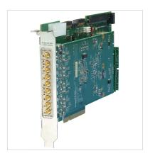
The Model 7890 generates up to eight synthesized clock signals suitable for driving A/D and D/A converters in high-performance real-time data acquisition and software radio systems. The clocks offer exceptionally low phase noise and jitter to preserve the signal quality of the data converters. These clocks are synthesized from onboard quad VCXOs (voltage controlled oscillators) and can be phase-locked to an external reference signal.
