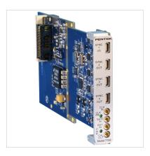
The Model 7192 High-Speed Synchronizer and Distribution Board synchronizes multiple Cobalt, Onyx, and Jade modules within a system. It enables synchronous sampling and timing for a wide range of multichannel high-speed data acquisition, DSP, and software radio applications.
