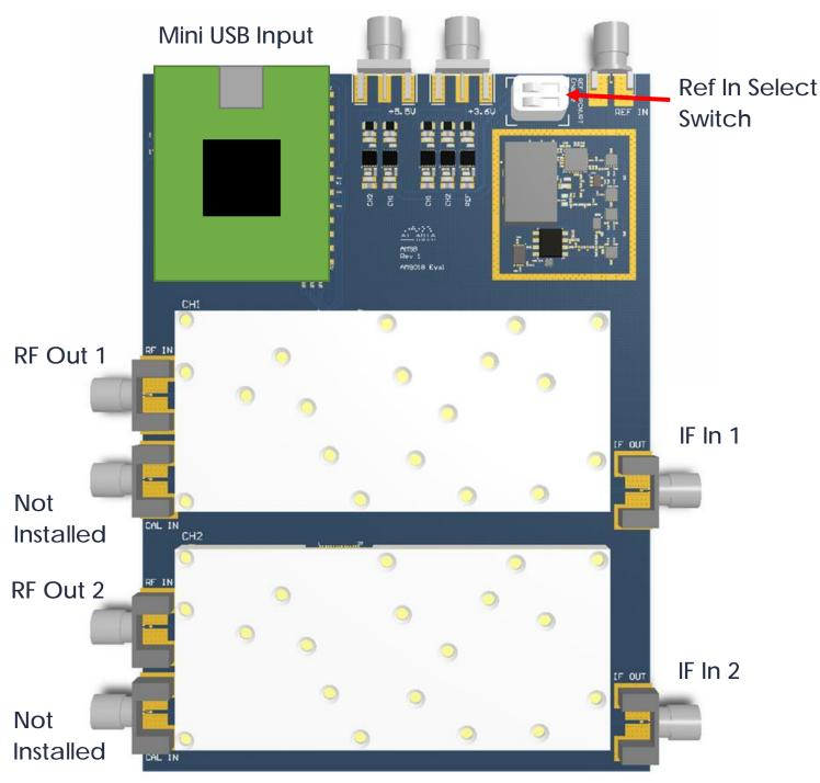
\*Note 1: Evaluation board supports up to two tuners to test phase coherent operation if desired.
