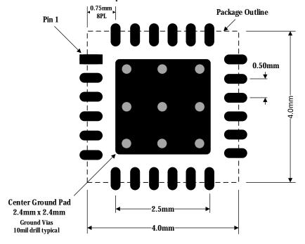
Pad and Spacing Detail 0.25mm
