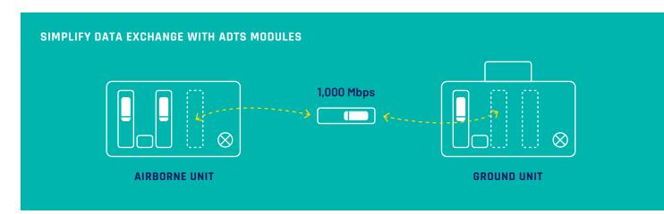
The ADTS simplifies data exchange and saves time with ground and airborne units that share a common design. Memory modules can simply be removed from the flight unit and inserted into the ground unit and vice versa. Operators do not need to move entire units to transfer data.
