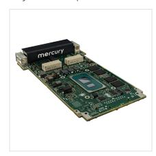
The first certifiable Intel Core i7 single-board computer with the latest-generation processor, the SBC3515-S delivers up to 40× better performance with built-in vector (AVX-512), Al accelerators, an Intel Gen12 Xe GPU and dual 10 GbE Ethernet.
