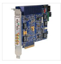
The 78630 is a high-speed data converter, suitable for connection to HF or IF ports of a communications or radar system. Its built-in data capture and playback features offer an ideal turnkey solution as well as a platform for developing and deploying custom FPGA processing IP.
