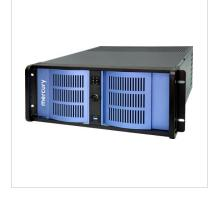
The Talon RTR 2745 is a turnkey, wideband recording and playback system that provides real-time capture of RF and IF signals. With two 3 GHz A/D converters and built-in DDCs, the system is ideal for capturing the IF outputs of RF downconverters with record-only bandwidths as high as 600 MHz. Selectable DDC tuning frequencies allow the RTR 2745 to accommodate a broad range of IF outputs.
