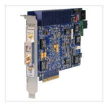
The 78641 is a high-speed data converter, suitable for connection to HF or IF ports of a communications or radar system. Its built-in data capture features offer an ideal turnkey solution. It includes a 3.6 GHz, 12-bit A/D converter and four banks of memory.
