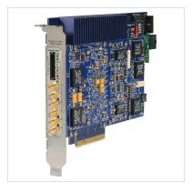
The 78651 is a two-channel, high-speed data converter with a programmable DDC, suitable for connection to HF or IF ports of a communications or radar system. Its built-in data capture and playback features offer an ideal turnkey solution.
