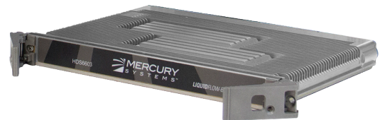
Figure 4: 6U OpenVPX Liquid Flow-By module
