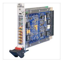
The 52671 is a 4-channel, high-speed data converter that is suitable for connection to transmit HF or IF ports of a communications or radar system. Its built-in data playback features offer an ideal turnkey solution for demanding transmit applications.
