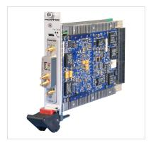
The 52640 is a high-speed data converter that is suitable for connection to HF or IF ports of a communications or radar system.
