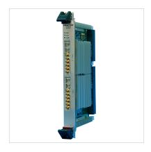
Cobalt 57671 and 58671 consist of one or two 71671 XMC modules mounted on a VPX carrier board. The 57671 is a 6U board with one 71671 module while the 58671 is a 6U board with two XMC modules rather than one.
