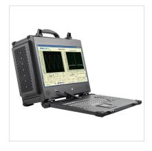
The Talon® RTR 2729A is a turnkey system that allows users to record very high-bandwidth signals in a lightweight and rugged portable package. Equipped with a 3.6 GHz 12-bit A/D converter and user-programmable DDC (digital downconverter), the RTR 2729A is capable of capturing RF/IF signals with bandwidths as high as 360 MHz continuously for more than four hours.
