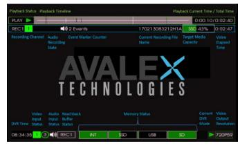
DVR ON-SCREEN DISPLAY (OSD) VIDEO OVERLAYS The DVR generates multiple horizontal status bars as onscreen overlays. These include a main status bar at the bottom of the display, a recording status bar for each record channel, and a playback status bar.
