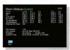
SYSTEM INFORMATION // The AVR8345 provides extensive system information by accessing the Status Menu, including memory, system, and logs. Shown here is the System submenu, which provides information on voltage, recorder runtime, and software version information.
