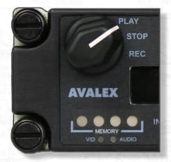
MODE CONTROL KNOB // The AVR8345 has a mode control knob that allows users to choose one of three modes:
