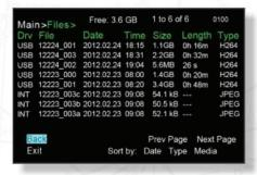
PLAYBACK // With the mode control knob on PLAY, files will automatically display on the monitor, allowing the operator to choose a file for playback. The file name, time played, total time, and file location are shown during playback.
