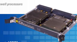
The EnsembleSeries™ GSC6202 accelerator is a 6U OpenVPX carrier module that integrates two high-performance NVIDIA GPGPUs for applications that can benefit from massively parallel processing on streams of high—bandwidth data delivering some of the highest GFLOP processing performance as well as the highest GFLOP/Watt performance efficiency in the industry.
