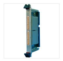
The 5790 and 5890 generate up to eight or 16 synthesized clock signals suitable for driving A/D and D/A converters in high-performance real-time data acquisition and software radio systems. The clocks offer exceptionally low phase noise and jitter to preserve the signal quality of the data converters. These clocks are synthesized from on-board quad VCXOs (voltage controlled oscillators) and can be phase-locked to an external reference signal.
