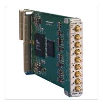
The Model 7190 generates up to eight synthesized clock signals suitable for driving A/D and D/A converters in high-performance real-time data acquisition and software radio systems. The clocks offer exceptionally low phase noise and jitter to preserve the signal quality of the data converters. These clocks are synthesized from onboard quad VCXOs (voltage controlled oscillators) and can be phase-locked to an external reference signal.
