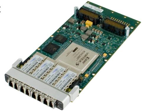
The Ensemble™ IO Mezzanine Series IOM-120 and IOM-140 (IOM-1x0) sFPDP XMC from Mercury Computer Systems brings enhanced performance and flexibility to external I/O in a serial RapidIO®-based streaming I/O XMC (Switched Mezzanine Card, VITA 42.2-2006). Providing 2.5 Gbaud of full-duplex bandwidth per channel and two or four channels per card, the IOM-1x0 Module offers high levels of speed and connection density.
