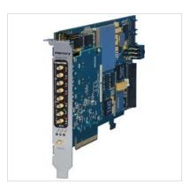
The Flexor® Model 7070 is a high-performance PCle board based on the Xilinx Virtex-7 FPGA. As a stand-alone processor board, it provides an ideal development and deployment platform for demanding signal processing applications.
