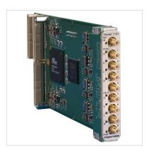
The Model 7191 generates up to eight synthesized clock signals suitable for driving A/D and D/A converters in high-performance real-time data acquisition and software radio systems. The clocks offer exceptionally low phase noise and jitter to preserve the signal quality of the data converters. These clocks are synthesized from onboard quad VCXOs (voltage controlled oscillators) and can be phase-locked to an external reference signal.
