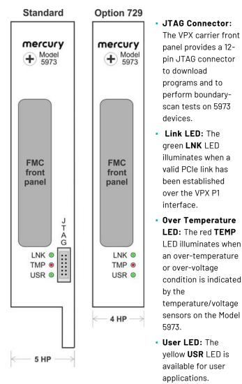
Note: If your 5973 is ordered with Option 763 for mounting in a conduction-cooled VPX chassis, it would have a conduction-cooled VPX Carrier Front Panel.
