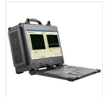
The Talon<sup>®</sup> RTR 2729A is a turnkey system that allows users to record very high-bandwidth signals in a lightweight and rugged portable package. Equipped with a 3.6 GHz 12-bit A/D converter and user-programmable DDC (digital downconverter), the RTR 2729A is capable of capturing RF/IF signals with bandwidths as high as 360 MHz continuously for more than four hours.
