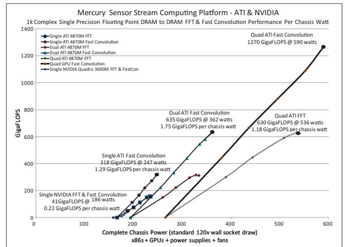
Figure 6. 1k Complex Single-Precision Floating-Point DRAM to DRAM FFT and Fast Convolution Performance per Chassis Watt
