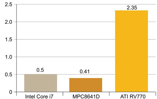
Figure 3. 1K Single-Precision Floating-Point FFT GFLOPS/Watt Performance
