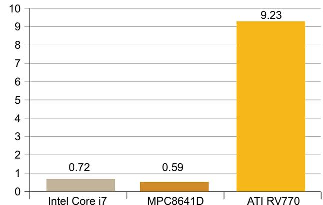
Figure 4. Peak Theoretical GFLOPS/Watt
