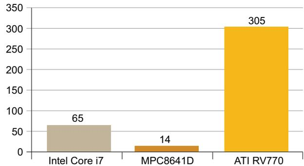
Figure 2. 1K FFT Single-Precision Floating-Point Performance
