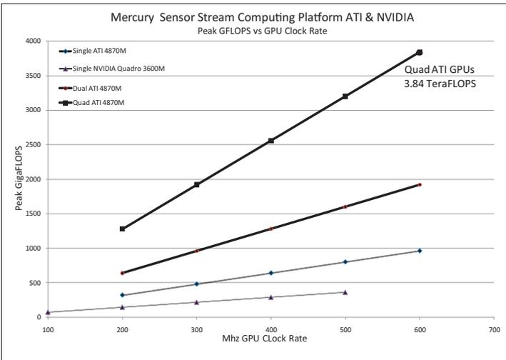
Figure 5. Peak GFLOPS vs. GPU Clock Rate in an SSCP System
