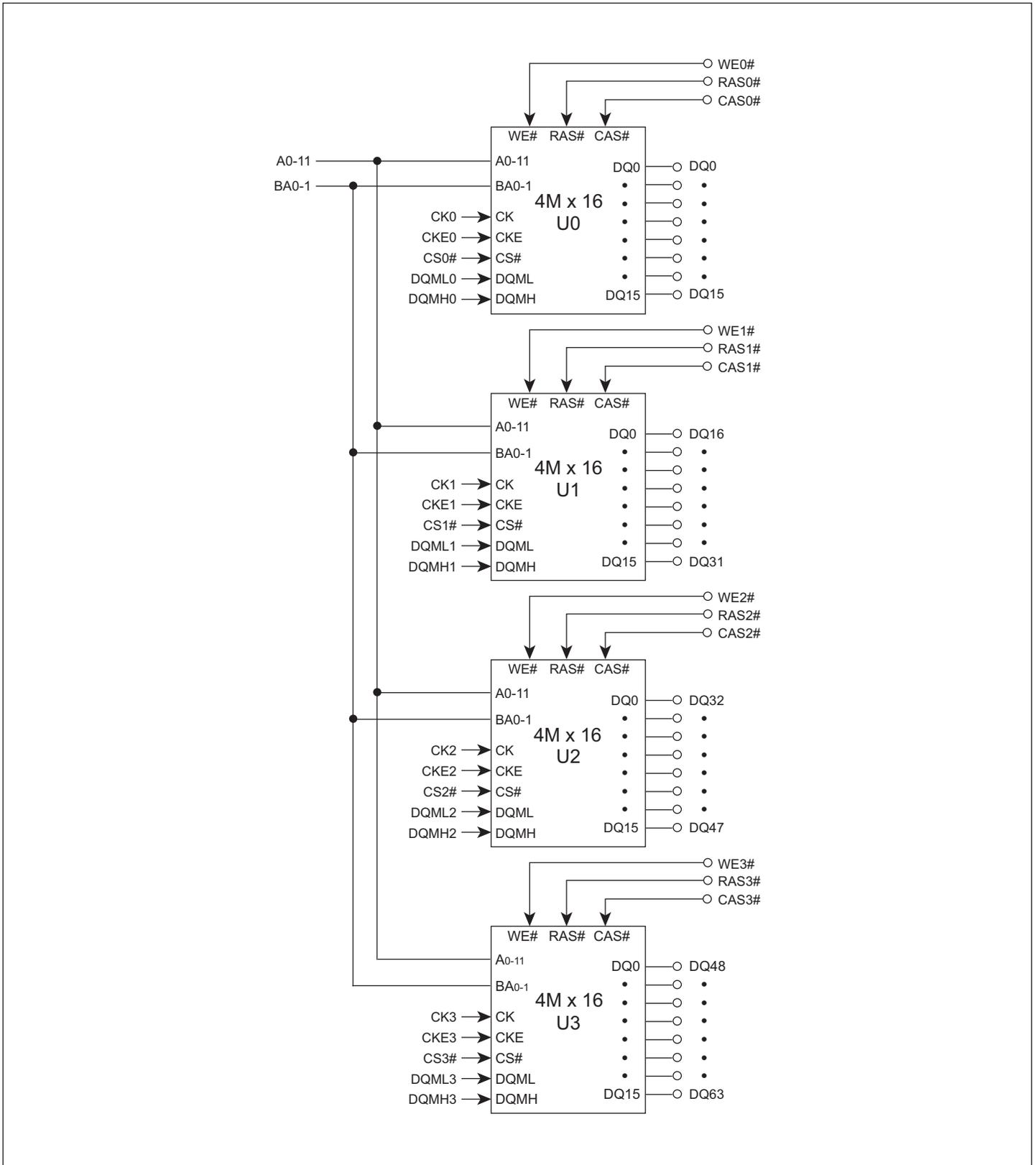
ability to synchronously burst data at a high data rate with automatic column-address generation, the ability to interleave between internal banks in order to hide precharge time and the capability to randomly change column addresses on each clock cycle during a burst access.
