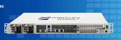
A part of the *EnterpriseSeries*", Mercury's RES-XR6 1U Server employs the latest Intel® Xeon® Scalable processors to accelerate compute intensive workloads for applications such as signal intelligence, cryptography, AI, surveillance, sensor fusion, analytics, communications, and audio/video processing.
