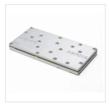
AM9018 is a fully integrated tuner module that provides high dynamic range coverage from 0.9 GHz to 18 GHz. The tuner also provides a bypass path from 10 MHz to 6 GHz for direct spectrum capture. The heterodyne tuner module is designed for high performance and low size, weight, and power (low SWaP) and is mechanically mountable to a host circuit board for use in multi-channel receiver applications.
