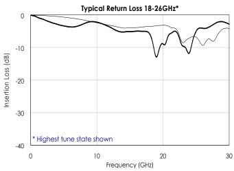
$<sup>^*</sup>$ Typical values shown for lowest tuned frequency (control bits 0000) or highest tuned frequency (control bits 1111)
