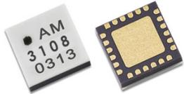
The AM3108 is a miniature digitally tunable highpass filter covering the 12.0 to 18.0 GHz frequency range. The filter provides 32 selectable highpass cutoff states with 5 digital control bits. The tunable lowpass filter can be combined with one of Mercury’s tunable lowpass filters to provide a flexible tunable bandpass filter solution. AM3108 has internal 50Ω matching, is packaged in a 4mm QFN package, and operates over the -40C to +85C temperature range.
