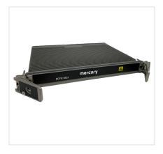
Mercury's SCFE6931 is a versatile OpenVPX heterogeneous processing module designed for high performance and agile system integration. Incorporating Xilinx's Versal® ACAP (Adaptive Compute Acceleration Platform) processors and advanced networking architecture, this advanced module maximizes application performance by combining scalar processing, vector processing and programmable logic into a single 6U design.
