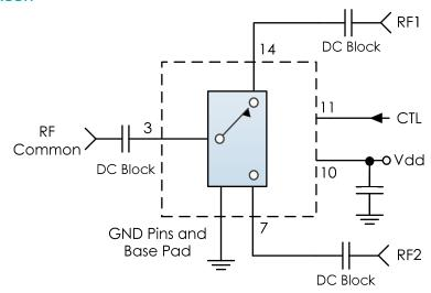
\*External DC blocking capacitors are required. Select capacitance values for low impedance across the frequency range of interest. See table below for CTL control information. NC pins may be left open or connected to ground.
