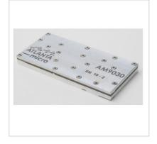
AM9030 is a fully integrated upconverter module that provides high dynamic range coverage from 0.9 GHz to 18 GHz. The upconverter also provides a bypass path from 10 MHz to 3 GHz for direct spectrum transmission. The heterodyne architecture is designed for high performance and low size, weight, and power (low SWaP) and is mechanically mountable to a host circuit board for use in multi-channel transmit applications.
