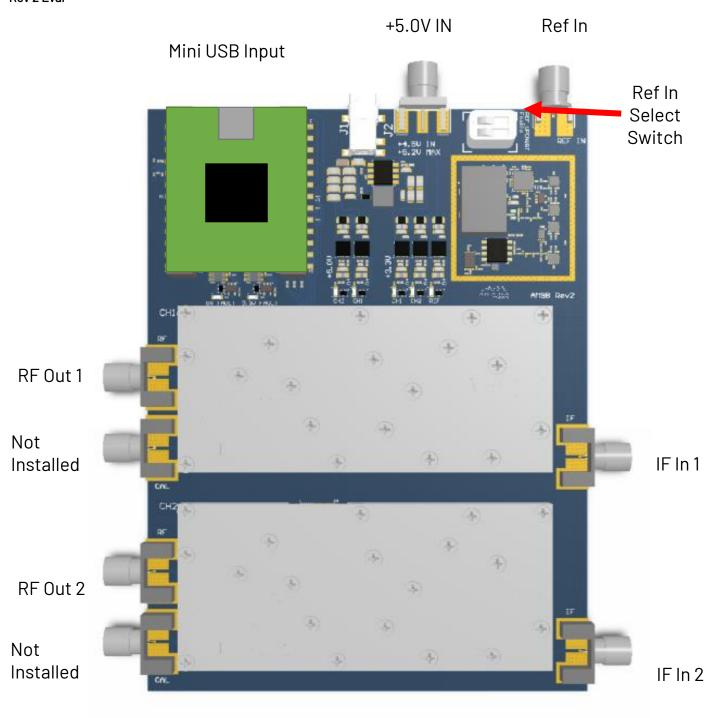
\*Note 1: Evaluation Board supports up to two tuners to test phase coherent operation if desired.
