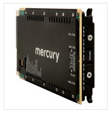
The DRF5580 is a high-performance, SOSA™ aligned 3U Open VPX board based on the Intel Agilex 9 Direct RF-Series. Four 64 GSPS A/D and D/A converters are integrated into the Agilex 9's multiprocessor architecture, creating a multichannel data conversion and processing solution on a single chip. The DRF5580 brings Agilex 9 performance to 3U VPX with a complete system on a board.
