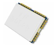
AM3073A is a shielded A/D driver module that provides amplification and antialiasing filtering of the 1.0 GHz IF output of the AM9017 tuner module. The AM3073A offers 500 MHz of bandwidth and 25 dB of gain packaged in an  $18 \text{mm} \times 24 \text{mm} \times 4.0 \text{mm}$  package while operating on +5.0V from -40C to +85C.
