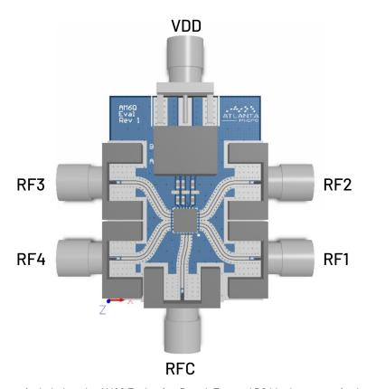
**Note:** DC blocking capacitors not included on the AM6Q Evaluation Board. External DC blocks are required.
