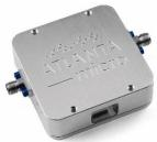
AM3023B is a miniature filter bank with 10 sub-octave filters covering the 100 MHz to 6000 MHz frequency range with full 80-MHz overlap from 400 to 6000 MHz available in a 20.5mm surface mount device or a USB controlled RF-shielded module.
