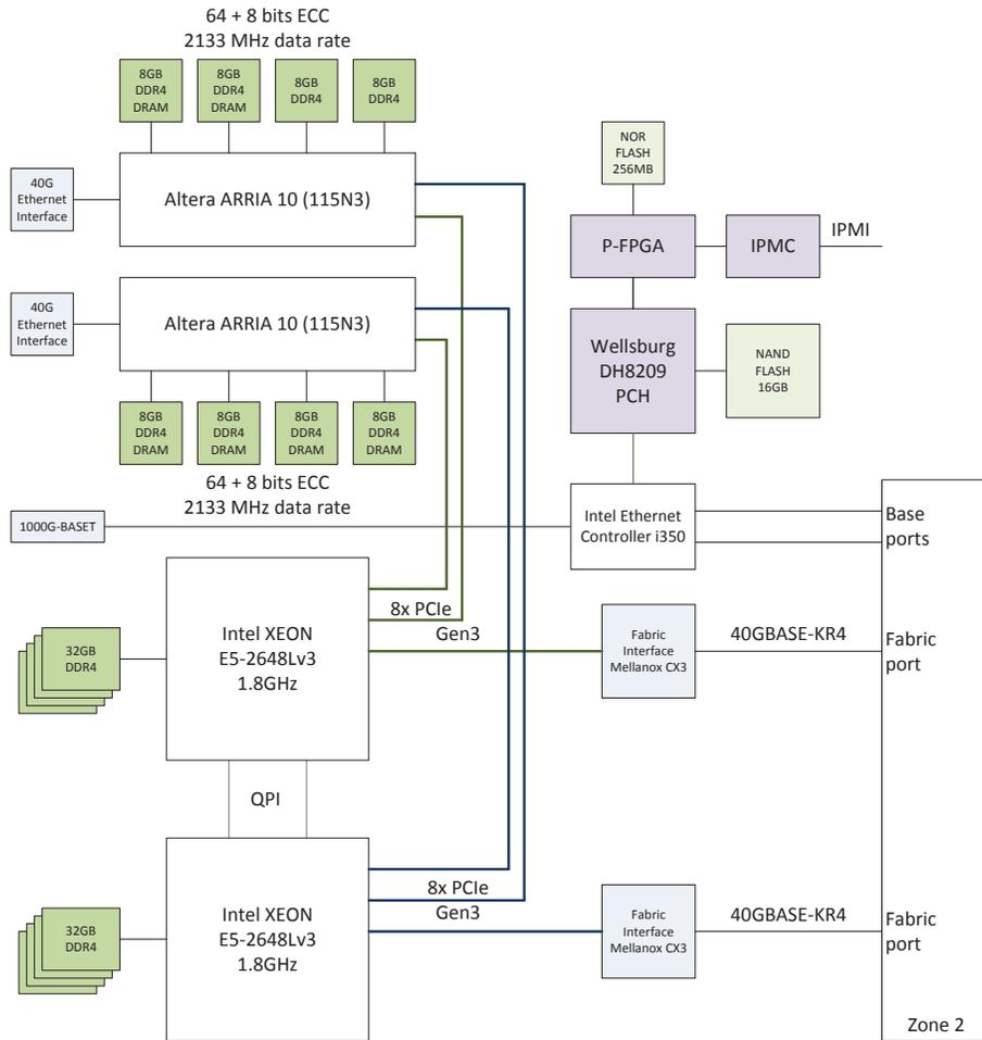
Figure 1: FCN8604 functional block diagram
