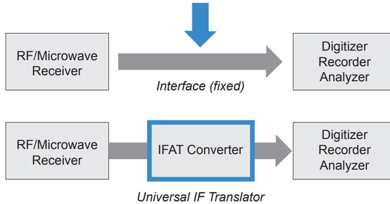
A "bridge" is necessary to keep up with these continuous changes and disruptions, adjusting the interface between your components as needs change over time or from project to project. The IFAT-2000 and IFAT-8000 fill that need.
