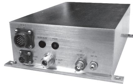
*Series BDC and BUC Block Converters enable frequency extension up to 40 GHz*
