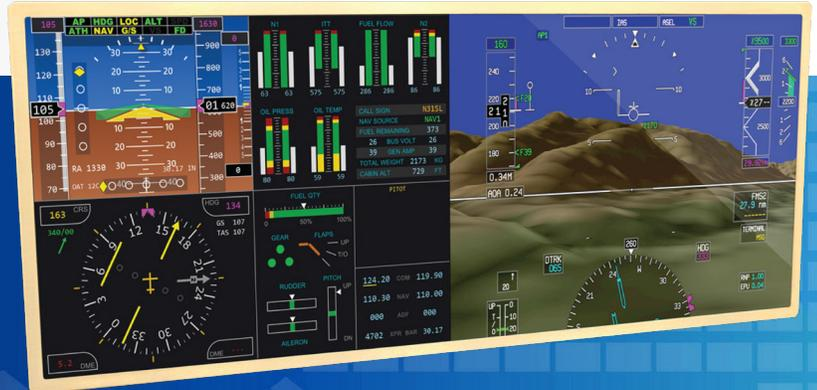
As the first dual-redundant large area display (LAD) of its kind, the LAD 2150 display head assembly (DHA) incorporates high-saturation color filters and 10-bit color depth affording a high-dynamic range of 1024 gray shades and capable of 1.3 billion colors.
