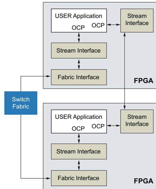
Figure 3. StreamFDK block diagram
