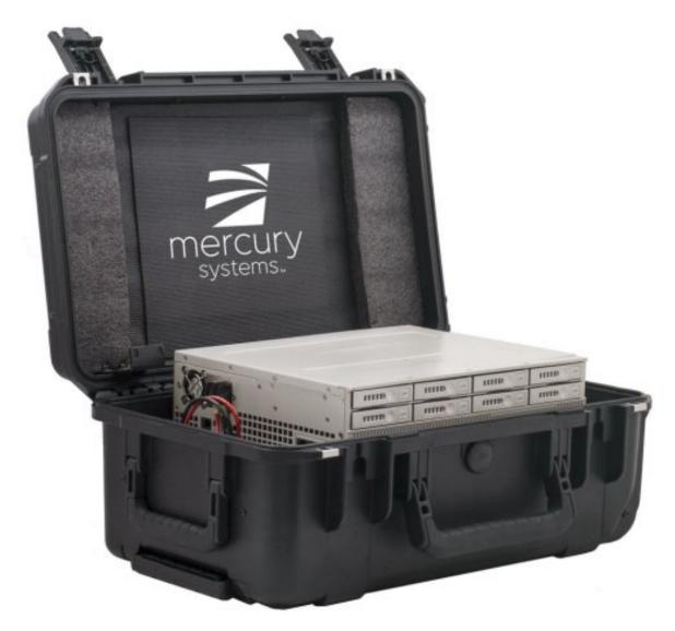
Mercury Systems calls its RESmini XR6 a data centre in a briefcase. The 6.8 kg server is designed to be mobile and rugged enough to operate in most stringent environments. (Mercury Systems)
