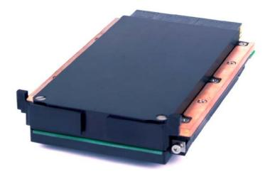
**TGA-300X** is designed for a wide variety of high performance graphics, video and GPGPU mission critical applications requiring flexibility in video input and output formats. Based on the AMD E4690, the TGA- $300X^{TM}$  has the latest graphics features and includes hardware acceleration of H.264, VC-1 High Definition video, as well as MPEG-2. Most of the processing is done in the GPU, off-loading the target system's CPU to maximize system performance.
