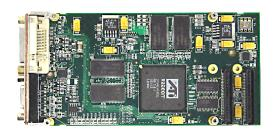
High Performance, Low Cost PMC 2-D Graphics Adapter with Dual-Display Support
