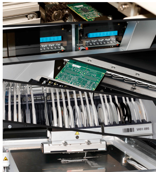
SMT component placement and automated component inventory carousels
