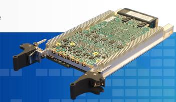
The DCM3220 digital transceiver is a multi-channel, highly configurable Rx/ Tx module with integrated FPGA processing. Optimized for high performance in SWaP-constrained environments, it offers low-latency, high instantaneous bandwidth and high analog input/output frequency. This versatile digital transceiver is available with rear I/O and is compliant to OpenVPX (VITA 65) to enable rapid system integration.
