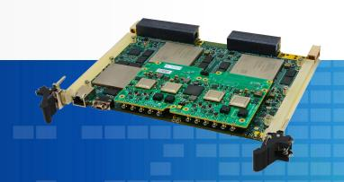
Mercury's EnsembleSeries™ DCM6222 is a versatile OpenVPX FPGA-based, Rx/Tx module designed for agile system integration and optimized to support system security engineering (SSE). This digital transceiver/ processor includes Virtex® UltraScale™ FPGA processing power, low-latency ADC/DAC performance and is ideal for operating in harsh environments. For a complete EW solution, the DCM6222 can be integrated with Mercury's ultra-wideband microwave transceivers, such as the RFM3101.
