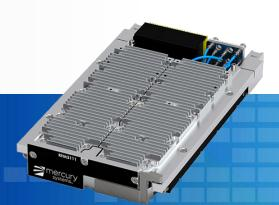
Mercury's SpectrumSeries RFM3111 is an ultra-wideband microwave transceiver with versatile local oscillator (LO), low-phase noise and fast tuning speed, packaged in a SOSA-aligned, low-SWaP 3U module. These versatile transceivers are open system architecture compliant and aligned in digital and RF processing domains through OpenVPX, OpenRFM, and SOSA.
